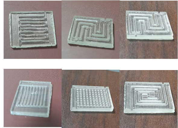
Fig. 5. 3D-printed test samples using a precise DLP machine right after printing.
