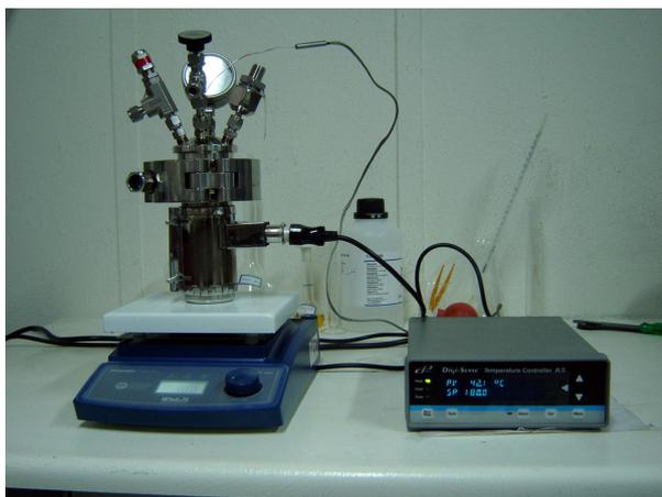
Fig. 2. The hydrothermal experimental setup.
