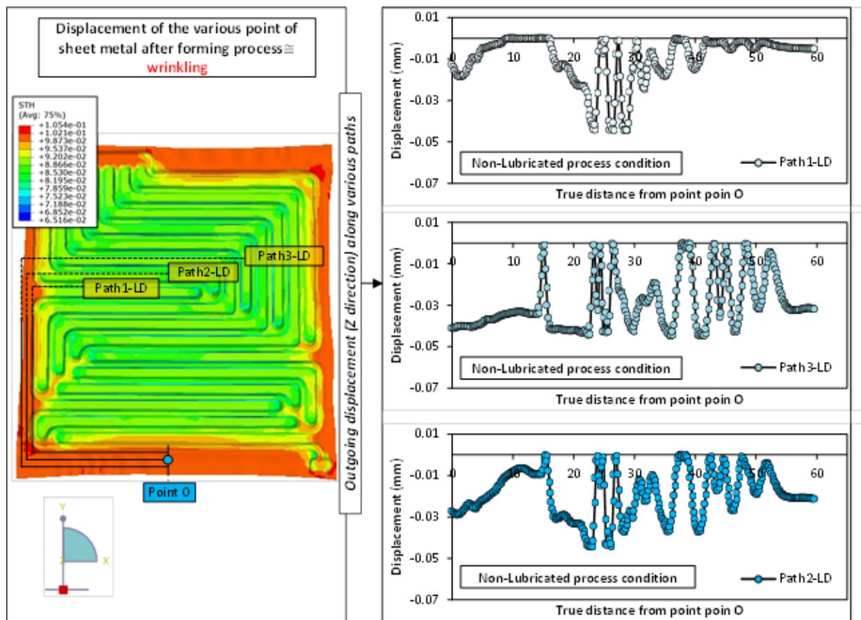
Fig. 4. The wrinkling of the left corner of the fabricated sample under non-lubricated conditions.
