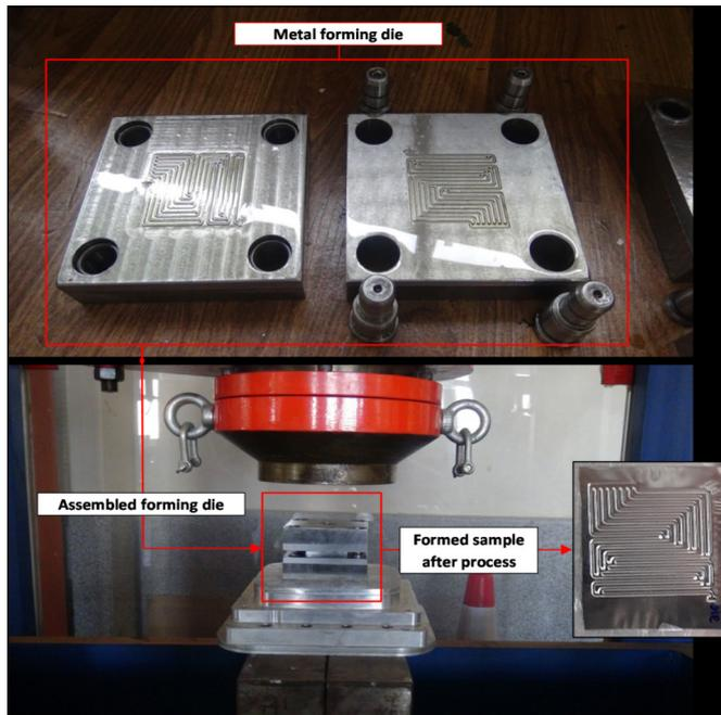
Fig. 1. The experimental equipment of the stamping process.
