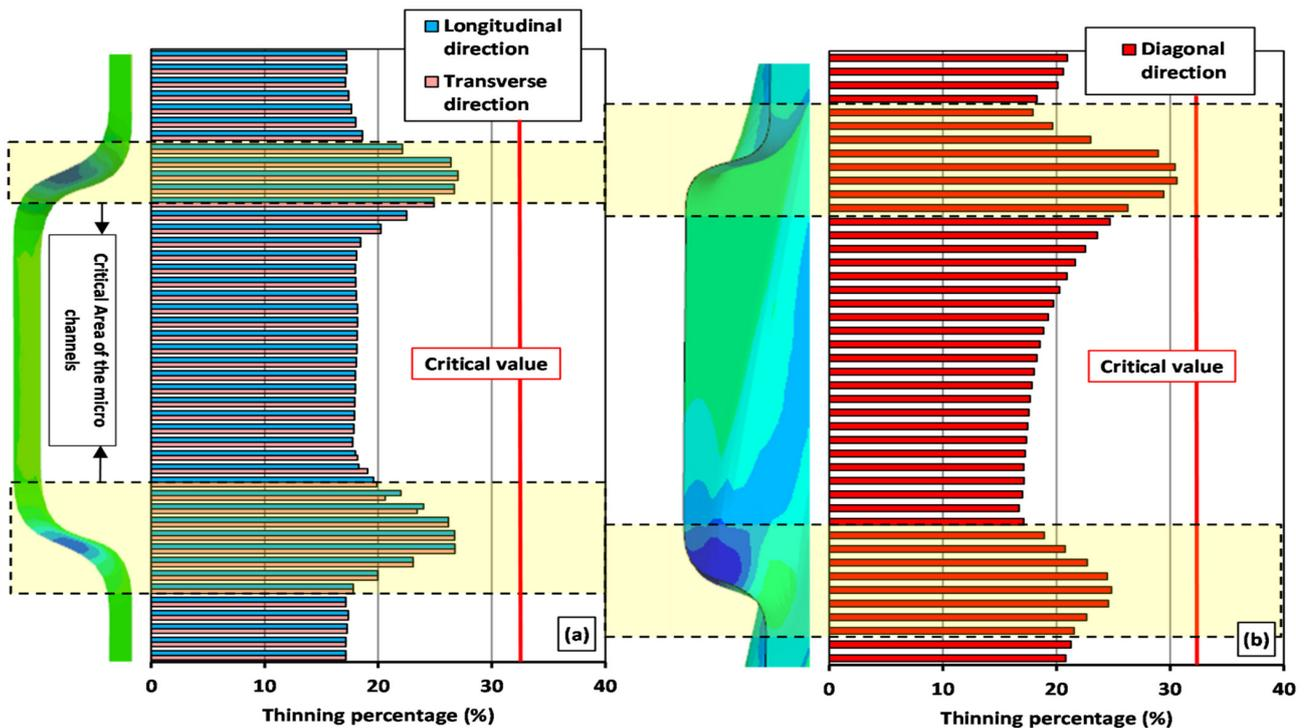
Fig. 3. Thickness distribution of MBPPs formed by the modified process together with the critical forming limit, a) transverse direction and longitudinal direction and b) diagonal direction.
