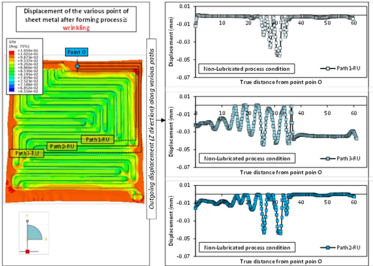
Fig. 5. The wrinkling of the right corner of the fabricated sample under non-lubricated conditions.
