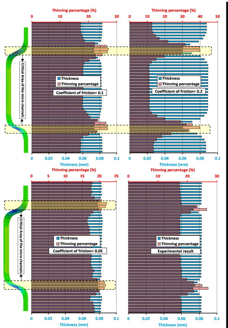
Fig. 2. Determination of the friction coefficient for the simulation of the SS316 bipolar plate forming process using a lubricant.
