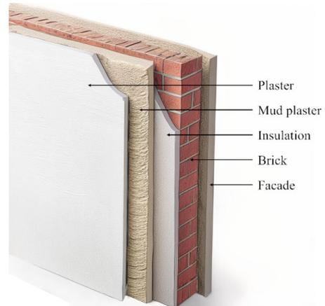
Fig. 3. Material composition of the external wall.
