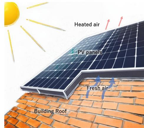
**Fig. 5.** Schematic of a BIPV/T system.
