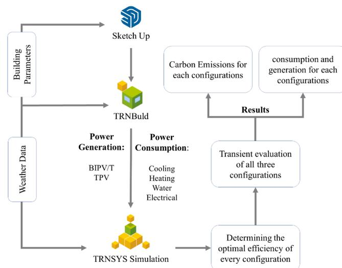
Fig. 6. Simulation process flowchart integrating 3D modeling with TRNSYS for transient analysis of building energy efficiency.
