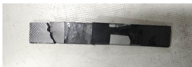
Fig. 4. Complete fracture of composite strips during lap shear testing.
