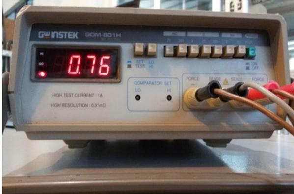
Fig. 4. Electrical resistance measuring device.
