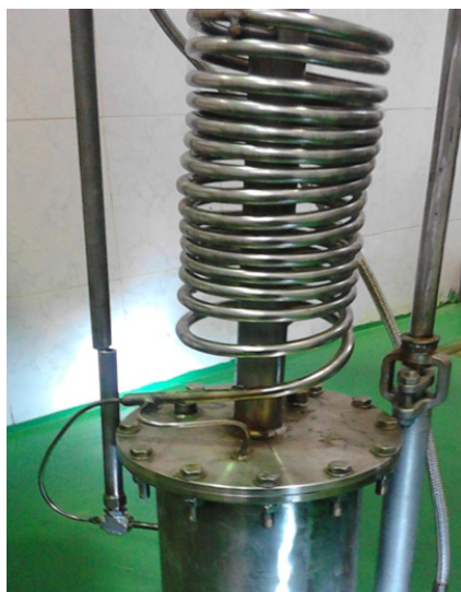
Fig. 5. Joule-Thomson cooling system manufactured according to simulation results.
