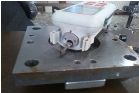
Fig. 4. Used roughness measuring device.
