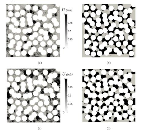
Fig. 4. Velocity and water distributions for: (a) & (b) a hydrophilic domain with the contact angle of 20; and (c) & (d) a hydrophobic domain with the contact angle of 150. Both domains are under the saturation of 0.5. The liquid water in (b) and (d) is shown in black while the air and the agglomerates are shown in gray and white, respectively.
