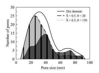
Fig. 5. The pore size distribution of the domain and the saturated pores in hydrophilic and hydrophobic domains.  $\overline{S}$  is the average liquid saturation of the domain.
