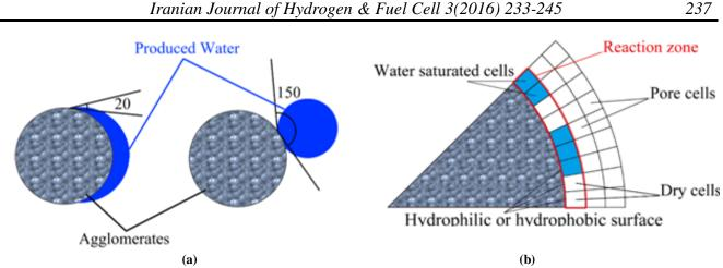
Fig. 1. a) The effect of contact angle on water formation at the surface of agglomerates. b) A schema of the cells applied in the numerical procedure.
