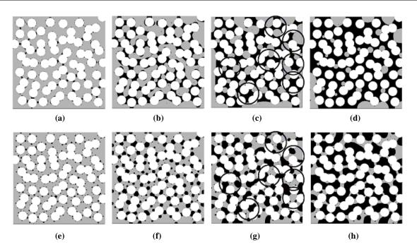
Fig.3. Water distribution for (a) - (d): a hydrophilic domain with the contact angle of 20; and (e) - (h): a hydrophobic domain with the contact angle of 150. Saturation is 0.10 in (a) and (e), 0.30 in (b) and (f), 0.50 in (c) and (g), and 0.70 in (d) and (h). The porosity of the domain is 0.50. The values of  $\alpha$  higher than 0.50 were shown for better visibility of liquid water which is in black. The gray area is air and agglomerates are shown in white.
