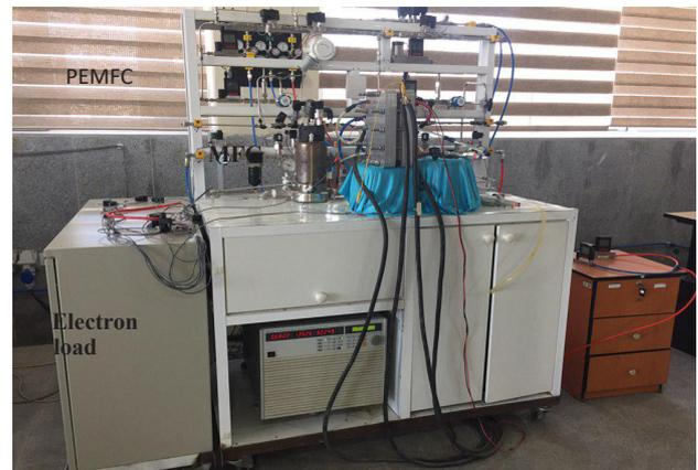
Fig. 3. Image of the PEMFC test station.
